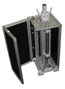
The PneuShock™ Model 9525C provides shock inputs for accurate and consistent sensitivity calibrations at high acceleration levels. Shocks are created at accelerations from 20g to 10,000g using a pneumatically operated projectile to strike an anvil and excite the sensor. By controlling both the level and the duration of the air pressure applied, the user gains greater control and consistency of the impacts. The system can be used manually in stand-alone mode or fully computer-controlled.
