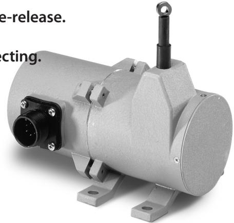
The patented Celesco Velocity Limiting System (VLS) is an option for PT8000 Series cable extension transducers that limits cable retraction to a safe 40 to 55 inches per second.
