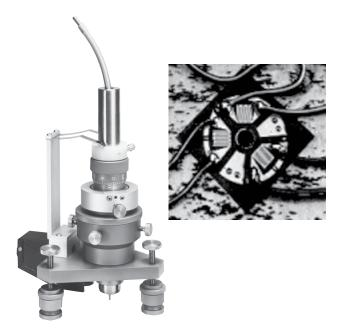
steel housing with eyepiece, reticle, and objective lens, permits alignment to within 0.0015 in (0.038 mm) of the gage center. The microscope is also used to measure the diameter of the hole after it is drilled. An illuminator attaches to the base of the guide to aid in the optical alignment procedure.
