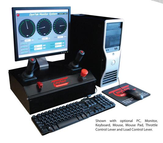
The DynTek-PC 2+2 engine dynamometer instrumentation system is a display only system intended for the most basic engine dynamometer testing requirements. This system provides for the measurement of torque in either tension or compression (both clockwise and counter-clockwise engine rotation), speed from a standard Magnetic Pickup along with two pressure and two temperature measurements.
